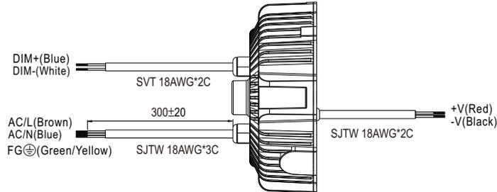
※ Built-in 3 in 1 dimming function, IP67 rated. Output constant current level can be adjusted through output cable by connecting a resistance or 1 ~ 10Vdc or 10V PWM signal between DIM+ and DIM-.
