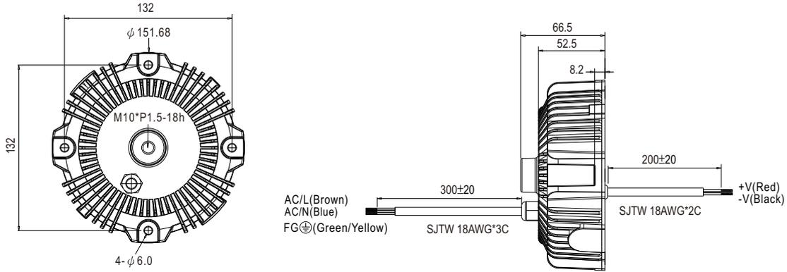
※IP67 rated. Cable for I/O connection.
