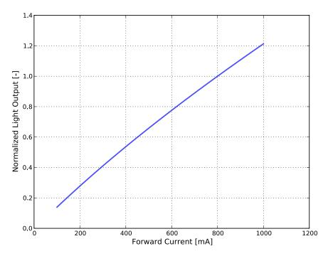
Figure 3c. Typical normalized light output vs. forward current for L150-xxxx5006000S0, T<sub>i</sub>=25°C.
