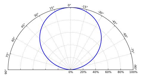
Figure 6. Typical polar radiation pattern for L150-xxxx50xx000x0 at specified test current, T<sub>i</sub>=25°C.
