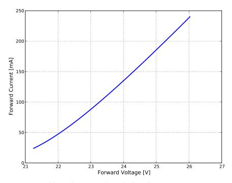
Figure 4a. Typical forward current vs. forward voltage for L150-xxxx502400000, T<sub>i</sub>=25°C.
