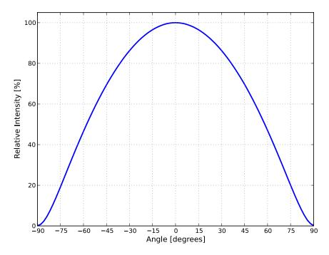
Figure 5. Typical radiation pattern for L150-xxxx50xx000x0 at specified test current, T<sub>i</sub>=25°C.
