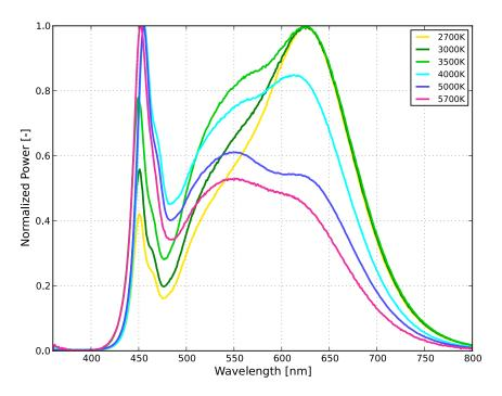
Figure 1c. Typical normalized power vs. wavelength for L150-xx9050xx00000 at test current,  $T_i$ =25°C.
