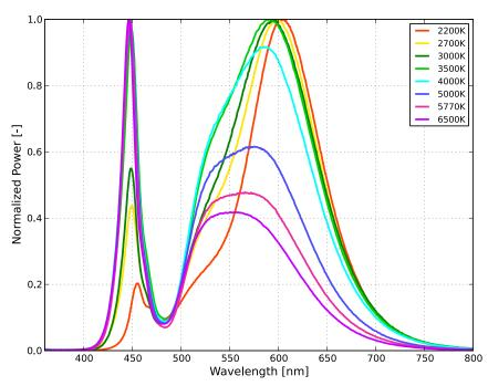
Figure 1a. Typical normalized power vs. wavelength for L150-xx7050xx000x0 at test current, T<sub>i</sub>=25°C.
