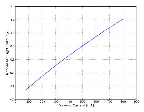
Figure 3b. Typical normalized light output vs. forward current for L150-xxxx500600000, T<sub>i</sub>=25°C.
