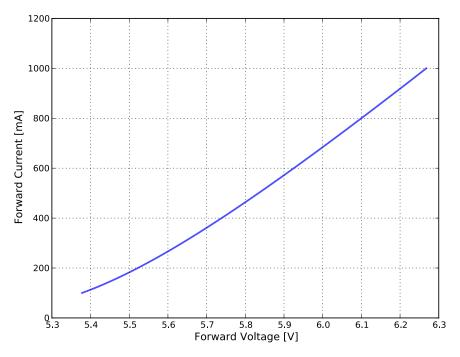
Figure 4d. Typical forward current vs. forward voltage for L150-xxxx5006000S0, T<sub>i</sub>=25°C.
