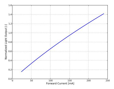
Figure 3a. Typical normalized light output vs. forward current for L150-xxxx50xx000x0, T<sub>i</sub>=25°C.
