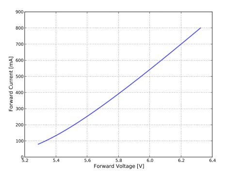
Figure 4b. Typical forward current vs. forward voltage for L150-xxxx500600000, T<sub>i</sub>=25°C.
