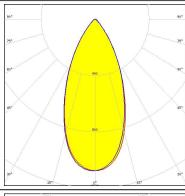
LED LC020C **FWHM** 25.0° 88 % Efficiency Peak intensity 2.5 cd/lm LEDs/each optic 1
