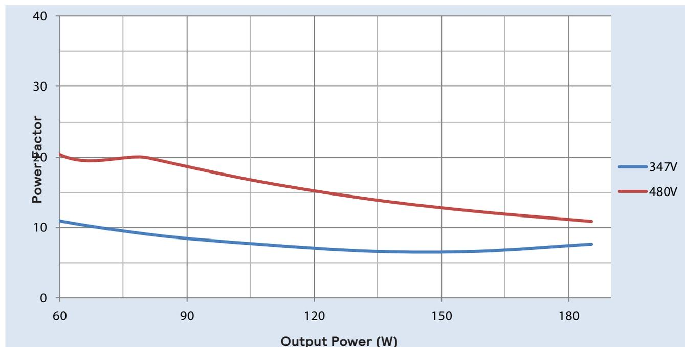
\* Power Factor and Total Harmonic Distortion graphs are shown for combined output power of both channels.
