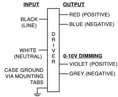
Input and output use lead-wires.
