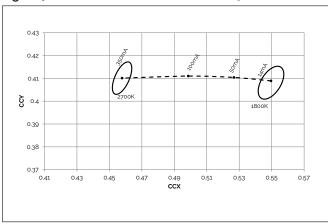
Figure 8: Color shift vs. Forward Current 3000K - 1800K
