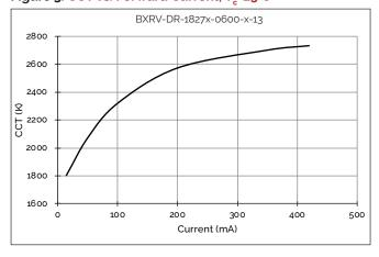
Figure 4: CCT vs. Forward Current, T\_=25°C
